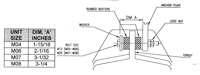
**Note: 1)** Tighten bolt to acheive dim. 'A'. This will pre compress the rubber buffers.
