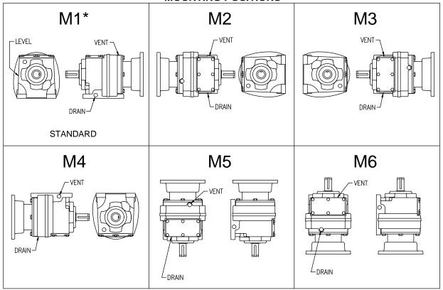
\* NOTE: The unit is filled at the factory with the proper amount of oil for the standard mounting position M1. A level plug is provided for this position only so the unit can be checked for proper oil level prior to installation and start-up. All other mounting positions will require the oil level to be measured out prior to filling the unit based on the values in the table labeled **OIL CAPACITIES** above.
