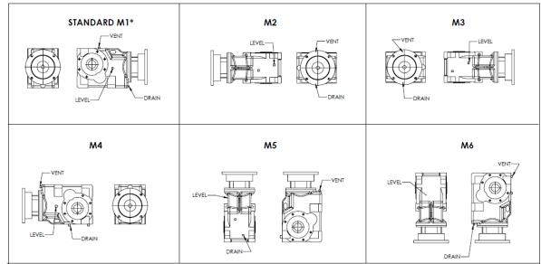
**NOTE:** The unit is filled at the factory with the proper amount of oil for the **STANDARD (M1)** mounting position. A level plug is provided for this position only so the unit can be checked for proper oil level prior to installation and start-up. All other mounting positions will require the oil level to be measured out prior to filling the unit based on the values in the table labeled **OIL CAPACITIES** above.
