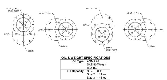
Before putting the unit into operation, substitute the vent plug for the solid plug at the position desired. Arrows indicate the recommended vent plug locations.
