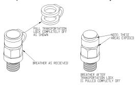
Before putting the unit into operation, it may be necessary to relocate the vent plug for positions other than standard (M1). Substitute the vent plug for the solid plug at the position desired. Install the solid plug in the location the vent plug was removed from. Refer to the following chart for the recommended vent plug locations based on mounting position
