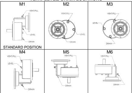
NOTE: The unit is filled at the factory with the proper amount of oil for the STANDARD mounting position. The level plug is for reference only so the unit can be checked for proper oil level prior to installation and start-up. All other mounting positions will require the oil level to be measured out prior to filling the unit based on the value in the table labeled OIL CAPACITIES below.
